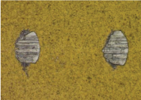
Figure 2. Sheared wire bonds.
