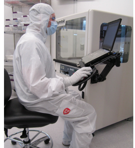
SMART's precision automatic dispense equipment.
