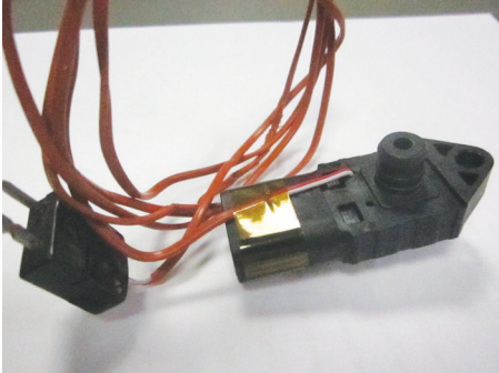
Figure 2. Thermocouple embedded into the gel of a specially modified part.
