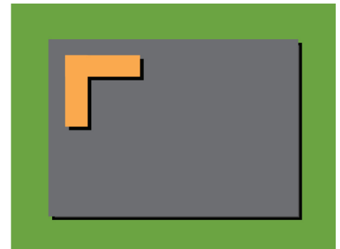
Die placement fiducial covered by die – can be assembled, cannot be measured after.
