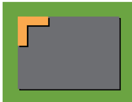
Die placement fiducial aligned with die – can be assembled, cannot be measured after.
