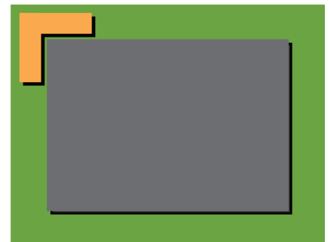
Die placement fiducial outside of die – can be assembled, can be measured after.
