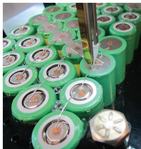
Figure 4. Aluminum wire on aluminum and nickel finishes.
