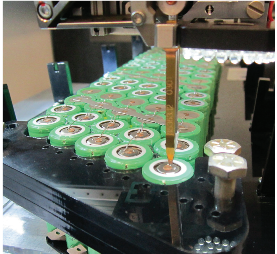
Figure 3. Close up of wire bond envelope – initiating first bond.
