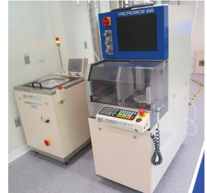
LoadPoint Wafer Dicing and Wash Station
